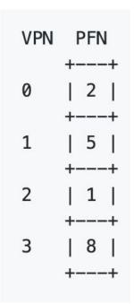
8-bit virtual address space, 10-bit physical address space, 64-byte pages
