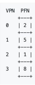
8-bit virtual address space, 10-bit physical address space, 64-byte pages
